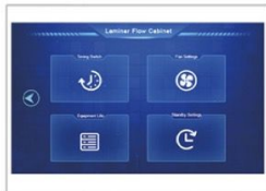
LCD Display 7-inch color touch screen, real-time display of running status.
